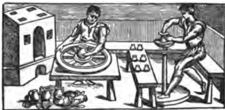
FIG. 5.—Two forms of Italian potter's wheels, about 1540.
